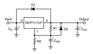
Figure 35. Protection Diode Placement
