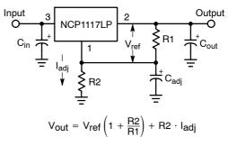
Figure 34. Adjustable Output Regulator
