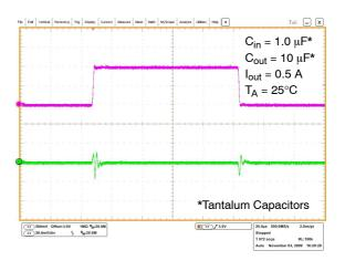
Figure 19. Line Transient Response – V<sub>out</sub> = 1.5 V
