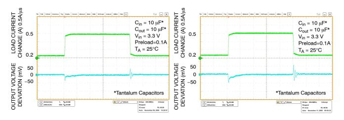
Figure 30. Load Transient Response – Vout = 3.3 V
