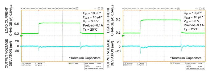
Figure 28. Load Transient Response – V<sub>out</sub> = 1.8 V
