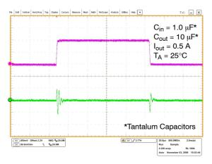
Figure 21. Line Transient Response – Vout = 1.8 V
