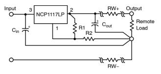
Figure 36. Load Sensing
