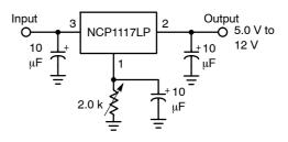
Figure 41. Adjusting Output of Fixed Voltage Regulators
