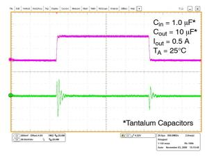
Figure 23. Line Transient Response – V<sub>out</sub> = 2.5 V
