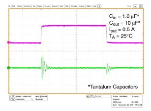
Figure 25. Line Transient Response – V<sub>out</sub> = 3.3 V
