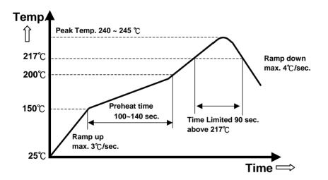
Note: The temperature refers to the pin of E48SR, measured on the pin +Vout joint.
