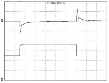
**Figure 8:** Output voltage response to step-change in load current (75%-50%-75% of lo, max; di/dt =  $0.1A/\mu$ s). Load cap: 10µF tantalum capacitor and 1µF ceramic capacitor. Top Trace: Vout (50mV/div, 200us/div), Bottom Trace: lout (5A/div). Scope measurement should be made using a BNC cable (length shorter than 20 inches). Position the load between 51 mm to 76 mm (2 inches to 3 inches) from the module
