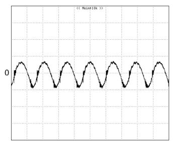
**Figure 11:** Input Terminal Ripple Current, *i*<sub>c</sub>, at full rated output current and nominal input voltage with 12µH source impedance and 33µF electrolytic capacitor (500 mA/div, 2us/div)
