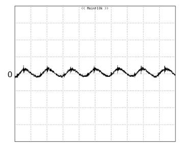
**Figure 12:** Input reflected ripple current,  $i_s$ , through a  $12\mu$ H source inductor at nominal input voltage and rated load current (20 mA/div, 2us/div)
