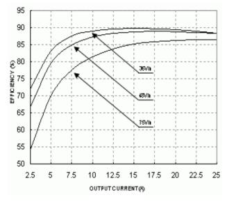
Figure 1: Efficiency vs. load current for minimum, nominal, and maximum input voltage at  $25^{\circ}$ C
