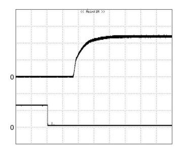
Figure 5: Turn-on transient at zero load current (2 ms/div). Vin=48V. Top Trace: Vout, 0.5V/div; Bottom Trace: ON/OFF input, 5V/div
