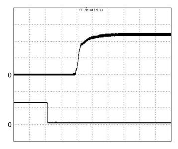
Figure 4: Turn-on transient at full rated load current (resistive load) (2 ms/div). Vin=48V. Top Trace: Vout, 0.5V/div; Bottom Trace: ON/OFF input, 5V/div
