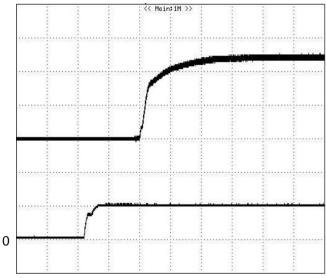
Figure 6: Turn-on transient at full rated load current (resistive load) (2 ms/div). Vin=48V. Top Trace: Vout, 0.5V/div; Bottom Trace: ON/OFF input, 5V/div
