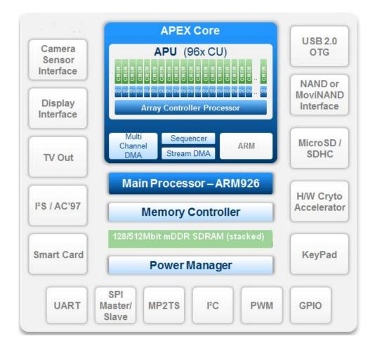
Figure 1. SCP 2200 Family Block Diagram
