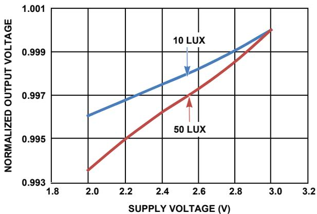
FIGURE 12. NORMALIZED OUTPUT VOLTAGE vs SUPPLY VOLTAGE
