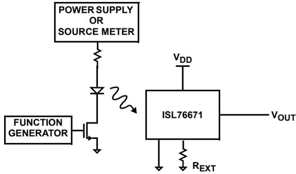
FIGURE 2. TEST CIRCUIT FOR RISE/FALL TIME MEASUREMENT
