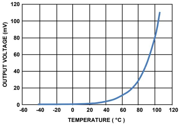
FIGURE 10. OUTPUT VOLTAGE vs TEMPERATURE AT 0 LUX
