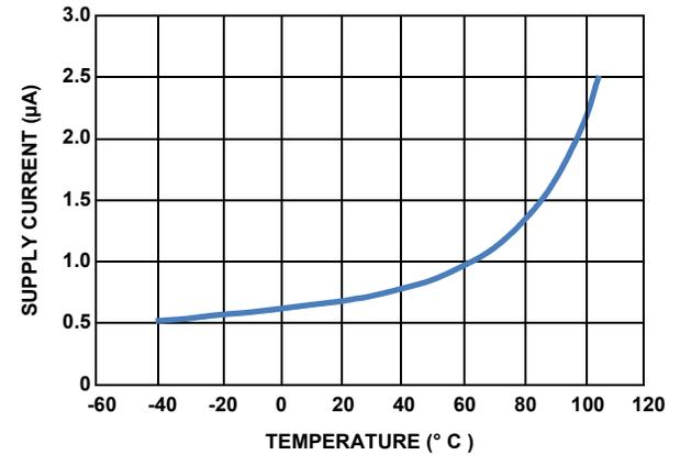
FIGURE 11. SUPPLY CURRENT vs TEMPERATURE AT 0 LUX
