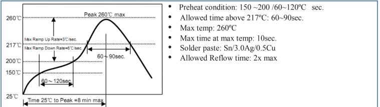
[Note: The reflow profile in the above table is only for qualification and is not meant to specify board assembly profiles. Actual board assembly profiles must be based on the customer's specific board design, solder paste and process, and should not exceed the parameters as the Reflow profile shows.]
