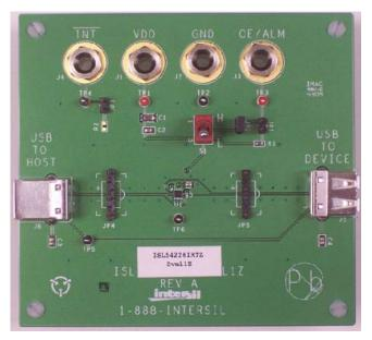
FIGURE 1. ISL54226IRTZEVAL1Z EVALUATION BOARD
