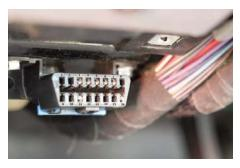
Data Link Connector in a 1998 Jeep Cherokee, with the pins labeled.
