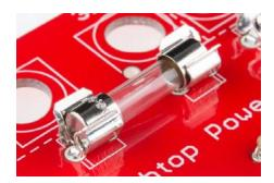
If the fuse slips out or won't stay inserted, take a pair of pliers and bend one side of the clip in towards the other. You'll want a good connection between the fuse clip and the fuse.
