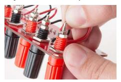
It is extremely important at this step to ensure you connect your wires tightly to the jacks and to clip of any dangling ends. We really don't want these to short out once the system is powered!
