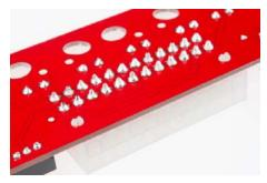
Make sure you insert the ATX connector all the way into the board before soldering it down. The two white tabs should pop through the guide-holes.
