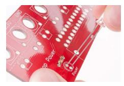
Make sure the LED is oriented properly before soldering it!
