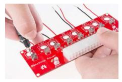
To connect your barrel jacks to your wires, you will want to unscrew the first small nut on the bottom of the barrel jack. Take the corresponding wire for that jack, and wrap it around the bottom of the jack. Then secure the wire in place by tightening back on the first nut to the jack.
