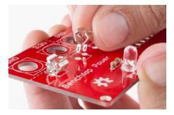
These can be a bit finicky at staying in the holes while you solder them, so it may help to bend the tab out a bit on each leg of the clip before attempting to solder them. Also, keep in mind that these are just basically hunks of metal, so they will take a lot of heat from the soldering iron to get a properly flowed joint. The clip itself will also heat up, so make sure you don't accidentally touch it and burn yourself!
