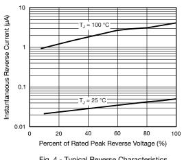
Fig. 4 - Typical Reverse Characteristics
