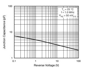
Fig. 5 - Typical Junction Capacitance
