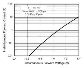
Fig. 3 - Typical Instantaneous Forward Characteristics
