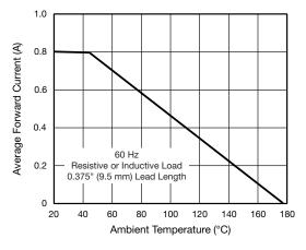
Fig. 1 - Forward Current Derating Curve
