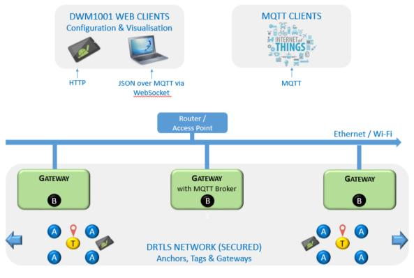
Figure 1: Target System Architecture
