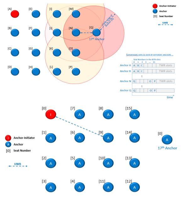
Figure 11: Scaling the DRTLS showing anchor's seat numbers
