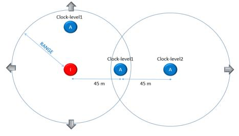
Figure 12: Scaling the DRTLS showing clock levels
