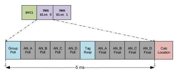
Figure 8: Superframe showing TWR frames
