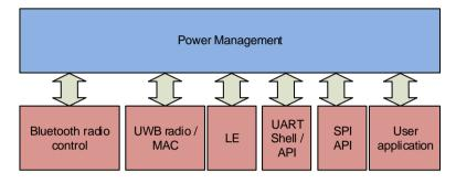
Figure 10: Main DWM1001 system components
