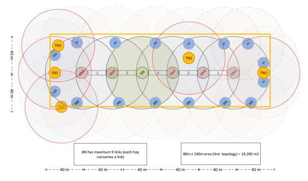
Figure 14: Single gateway area coverage with line topology
