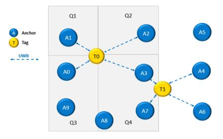
Figure 9: Tags choice of anchors for TWR
